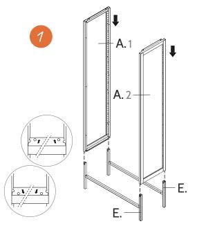
Attention: Holes must face outwards, plastic levelling feet must face down.
