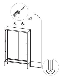
Is the surface uneven? Turn the plastic levellingfeet to correct this.
