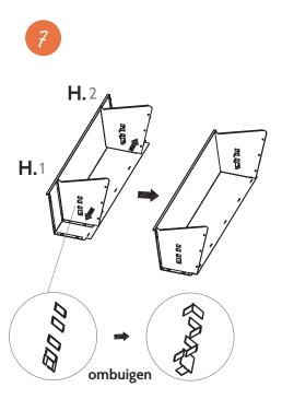
Not using dividers? (step 10) then do not bend the tabs.
